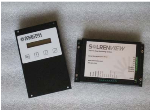
Solrenview Lite Residential & Solrenview LCD, advanced version great for larger multi-inverter systems
