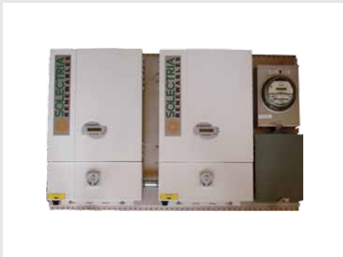
The double integrated panel option for PVI 3000-7500 includes inverters, back panel, AC subpanel with breakers, integrated DC disconnects and revenue grade meter.
